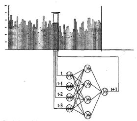
Fig. 1. Neural Network application to time series forecasting with a (4-4-1) MLP, using n=4 input neurons for observations in t, t-1, t-2, t-3, four hidden units, one output neuron for time period t+1 and two layers of 20 trainable weights. [23]
